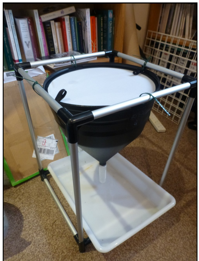
Figure 1. Standard Berlese Funnel manufactured by BugDorm. © Richard Wilson.
