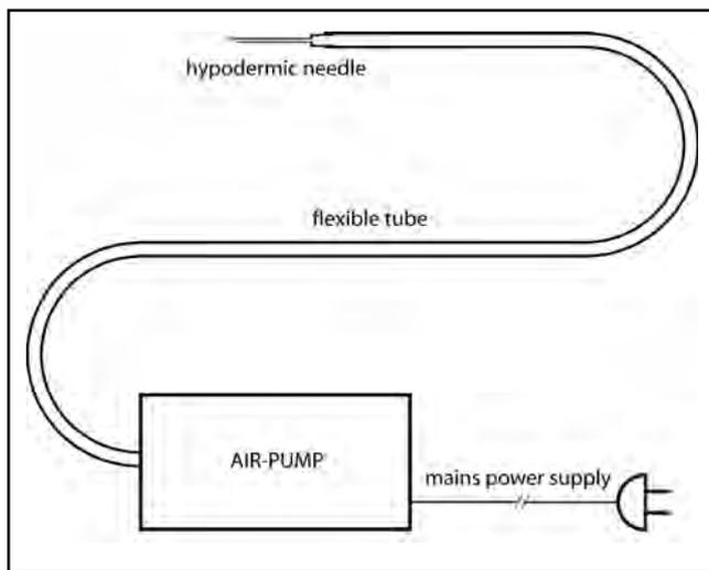
Figure 1. Diagram showing construction of the Aeronneedle.
