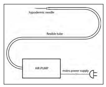
Figure 1. Diagram showing construction of the Aeroneedle.
